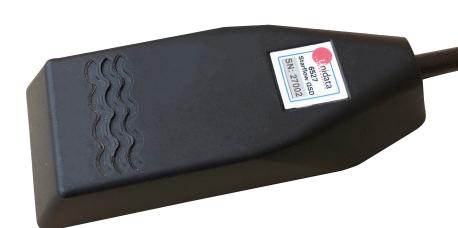
The Unidata 6527 Starflow QSD SDI-12 Instrument is used to measure water velocity, depth and temperature of water flowing in rivers, streams, open channels and large pipes. When used with a companion Unidata IP data logger, flow rate and total flow can also be calculated.
